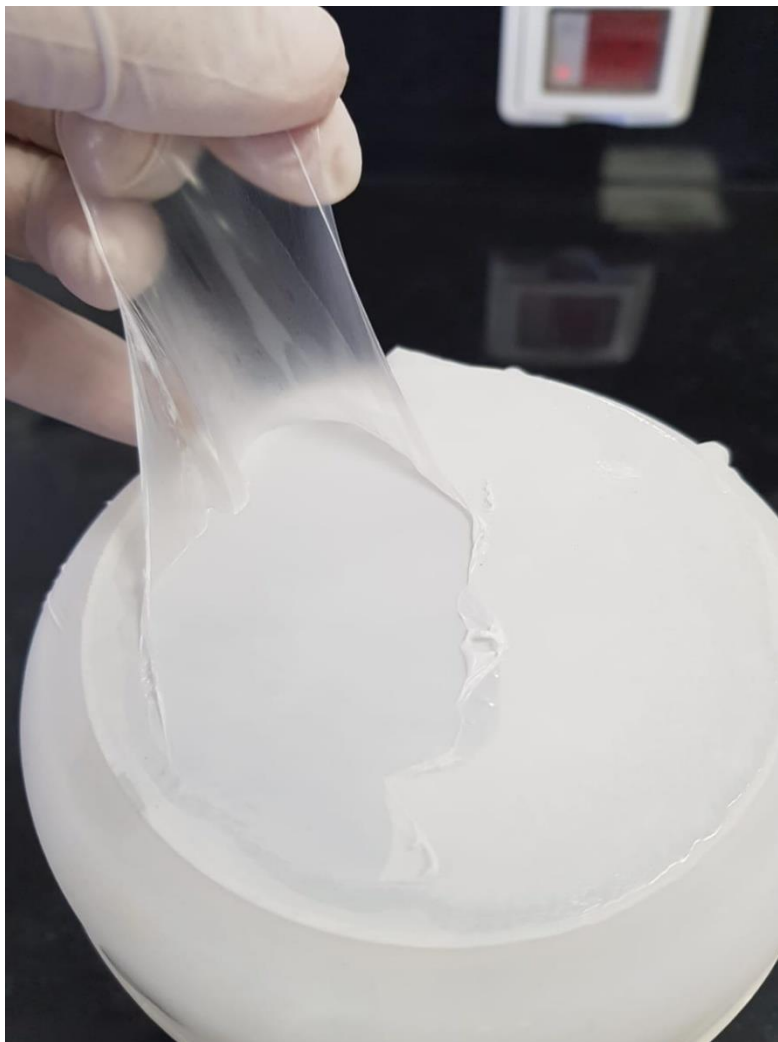
Figure #21. Removing thin film applied on rubber surface after washing with water.
