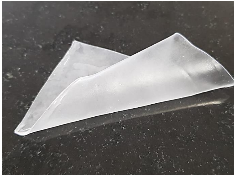
Figure #20. Thick film (D4) was rolled up to assess its flexibility.
